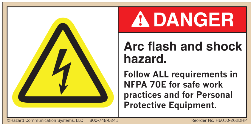
Fig. 2. A warning label must be placed on any piece of electrical equipment that may remain energized during maintenance or repair.
