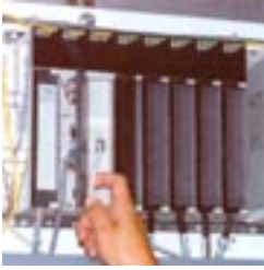
Schneider Automation Ethernet TCP/IP module and category 5 Ethernet cable.
