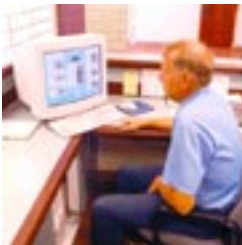
Water treatment plant operator checks the SCADA Operator HMI's main screen. This terminal is one of four Pentium PCs that reside as independent nodes on the Ethernet network.
